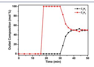
**Figure 7.** Experimental data on transient breakthrough of an equimolar  $C_2H_4/C_2H_6$  mixture in an adsorber bed packed with PAF-1-SO<sub>3</sub>Ag in the adsorption phase of a PSA operation.
